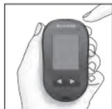
Pulse y suelte
